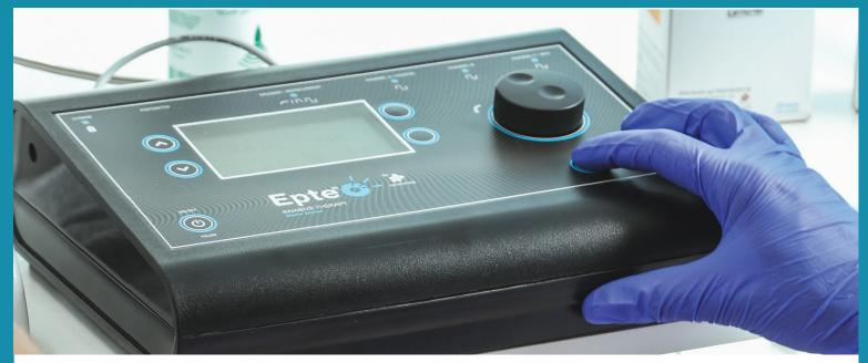
The EPTE Bipolar System (EPTEV02V01) device is composed of three current sources (A, B and C) monophasic/biphasic, capable of generating constant currents (galvanic), pulsed monophasic and biphasic currents (symmetric/asymmetric), whose application is used for different treatments of pathologies of the musculoskeletal system acting on this or the central or peripheral nervous system depending on the applied therapy.
